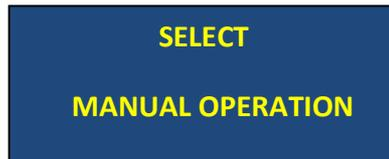
Pressing “ENT” button on this screen will put the controller in Manual mode. This mode will continue to run till it is purposefully changed or Power down. This mode is normally used to perform the operation like:
